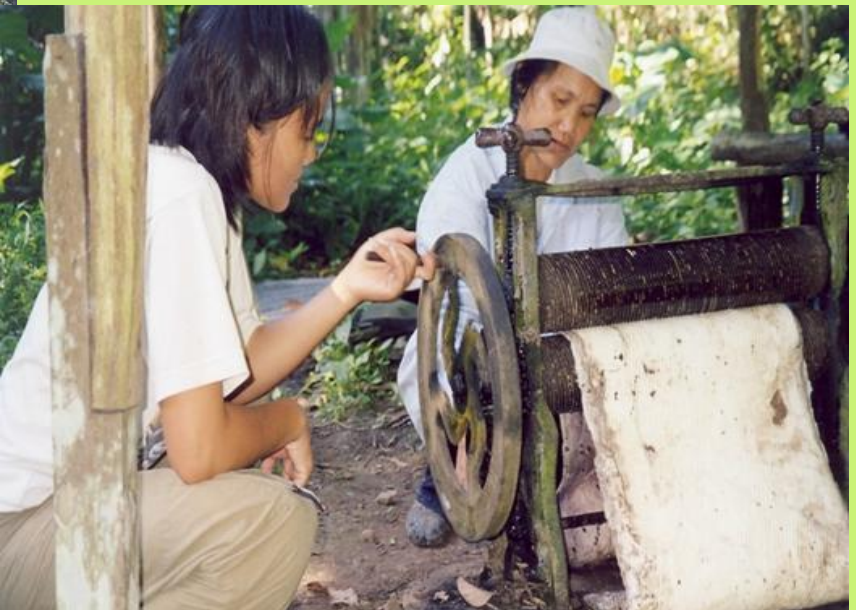
Rubber sheets being pressed
